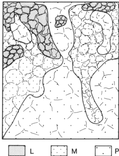
Fig. 2: Schematic representation of a polished face in the central part of an undisturbed indurated sample, taken from photo 6.
